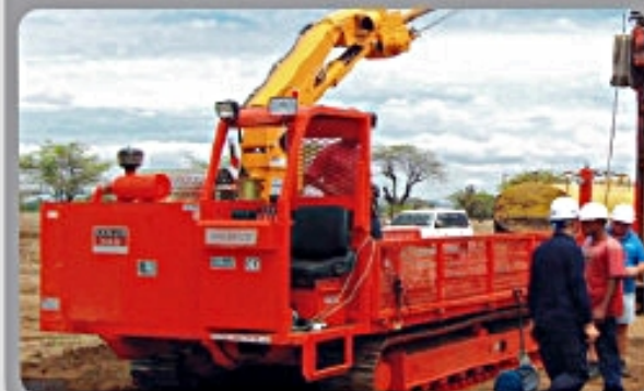
D&B 10CR-03 (3ton crane)
